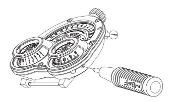
To adjust the date, gently position the supplied tool in the corrector hole, which is located on the right-hand side of the case.
